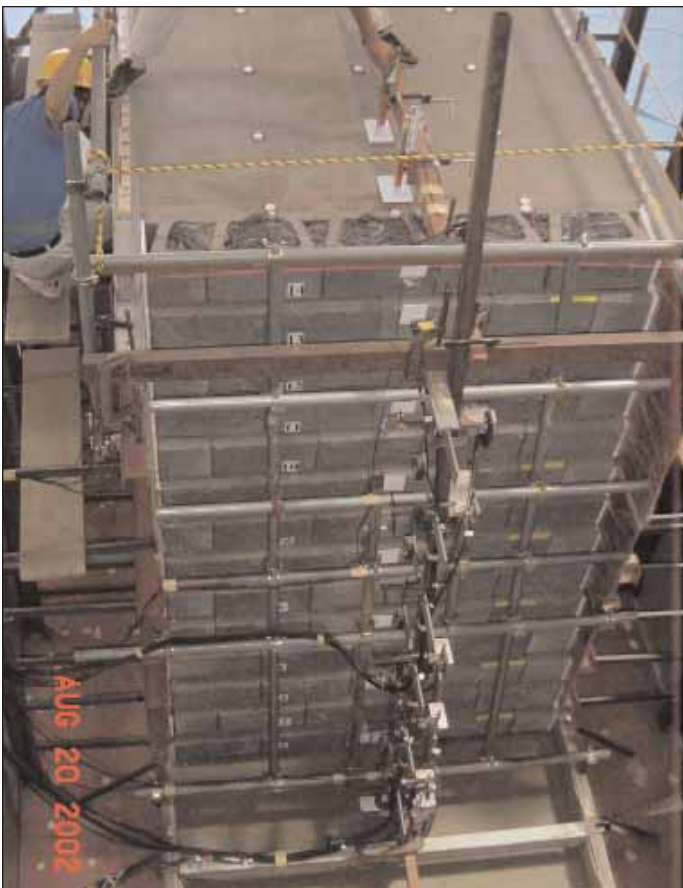
Completed Structure on Shake Table
